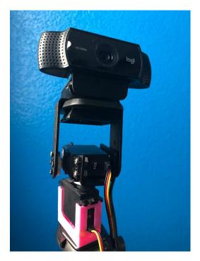
Fig. C1. Servo Stand with Tripod [42]
