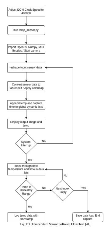
The chart above in Fig. B3 summarizes the process of the operation of the thermal camera sensor. The temperature begins its operation by adjusting the system's i2c-0 bus clock speed and terminates when the index of temperature data is empty. The program saves a data log at termination of the software.
